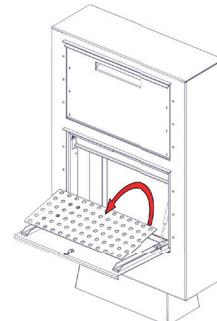
4. Mark the position of the holes at the bottom of the parcel letterbox on the paving slab or surface.
