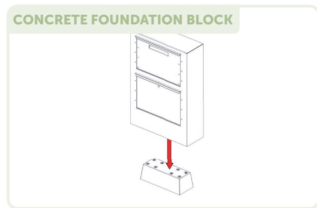
8. Secure the parcel letterbox to the paving or paving stone using plugs or chemical anchors. This is not necessary when securing to a concrete base.
